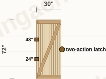
RUN DOOR — VIEWED FROM THE BACK
