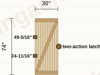
RUN DOOR — VIEWED FROM THE BACK
